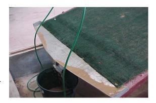
Sediment loss is calculated by determining the water (w) to sediment (s) ratio (w/s) of the sediment samples by dividing the dry sample weight by the original sample weight. This ratio is applied to the full sediment sample to determine total sediment loss.
