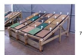
Vegetation cover is based on the average percent of surface cover achieved in three standard nursery flats (12 in x 18 in) covered with the selected Class 1 material. Flats are seeded with the seeding mixture, placed on 3:1 and 2:1 racks and allowed to grow for 90 days. Percent vegetation covered is determined using a digital camera and processed using the current VCAP technology.
