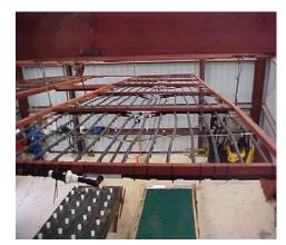
Rainfall simulation is done using a new simulator that more closely reproduces the more damaging precipitation drop sizes found in more intense storms. Uniformity of the coverage and precipitation rate are carefully controlled. Each test consist of three (3), repetitions of three, 30-minute storms of 3.5 in/hr. After each set of 3 rainfall events, the test bed is completely rebuilt with new soil and new Class 1 material.
