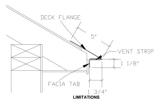
**Inland II:** Do not install this product on buildings with a mean roof height greater than 50 feet. **Inland I:** Do not install this product on buildings with a mean roof height greater than 33 feet. **Seaward:** Do not install this product on buildings with a mean roof height greater than 33 feet.
