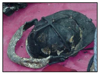
became disoriented and escaped the building with serious burns. All three were wearing full NFPA-compliant protective ensembles and SCBA. The helmets of the two most seriously burned firefighters, Chapa and Haynes, showed evidence of extreme heat exposure, with face shields burned and deformed, but helmet shells, although burned, were intact.
