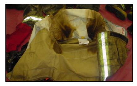
The fabric shells of Haynes' Chapa's and bunker gear showed extensive melting to reflective trim. Inner liner barriers vapor were scorched even though the fabric shells of the coats appeared undamaged other than damage to the reflective trim.
