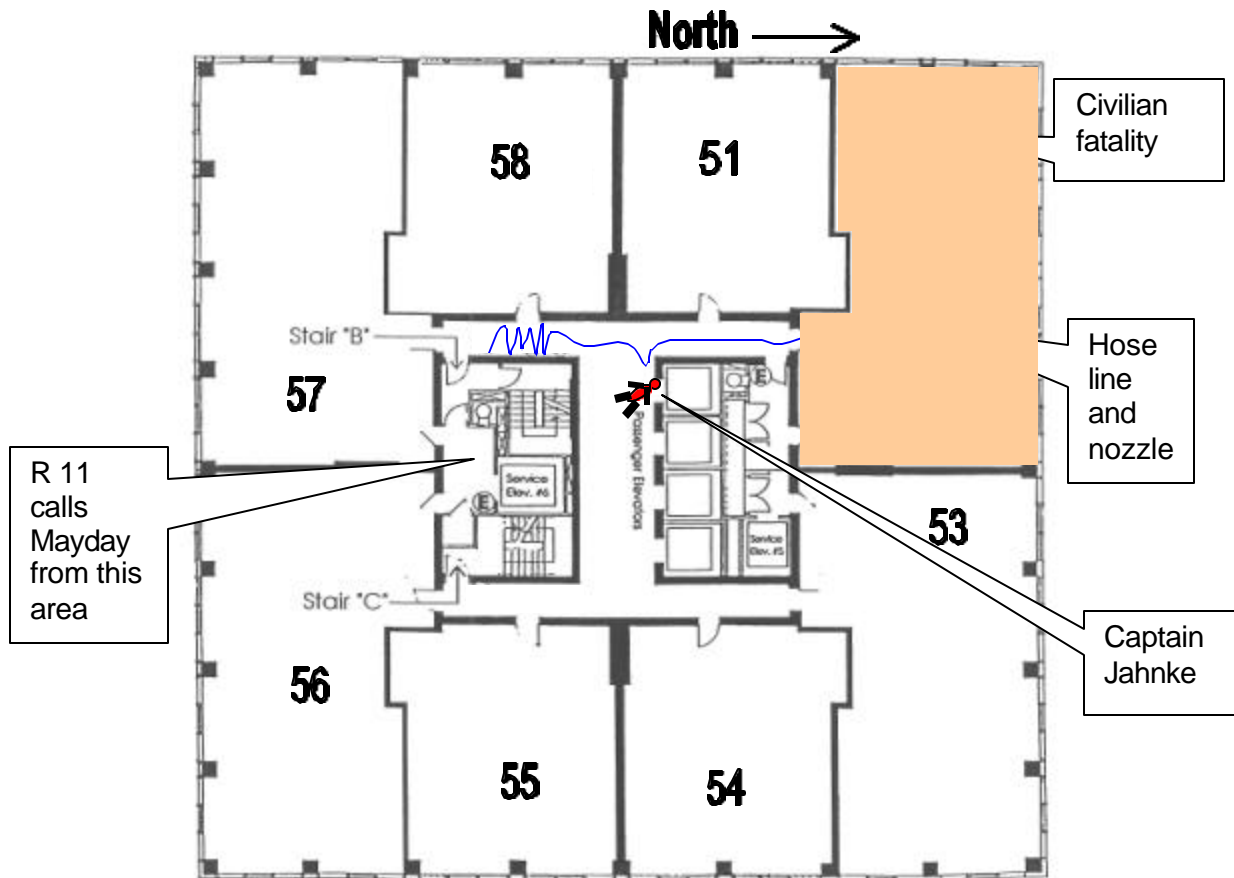
Figure 13-Fifth floor layout. Locations of civilian victim, Captain Jahnke, and fire hoseline are approximate and based on firefighter interviews.
