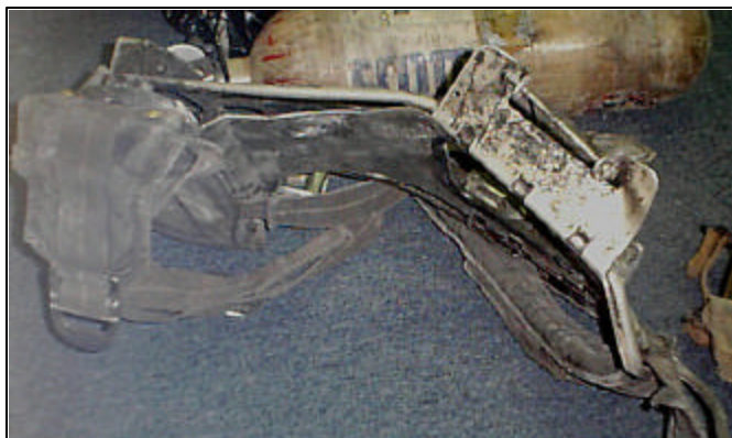
Figure 15. Bent SCBA backpack assembly.
