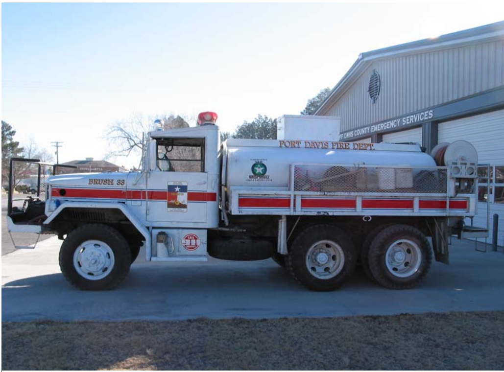
Figure 15 - 1970 Kaiser Brush Truck – 350 GPM Pump, 1200 gallons of Water, (Brush 33)
