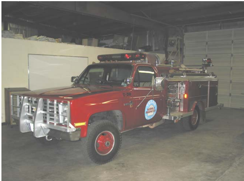
Figure 7 – Mini-Pumper –1985 Chevy; 250 GPM Pump, 300 gallons of water, pump has not been tested, carries 250' of 2 ½" hose, unit is considered the “front line” attack truck for structure fires and lacks adequate equipment for what would be considered a Class A Engine
