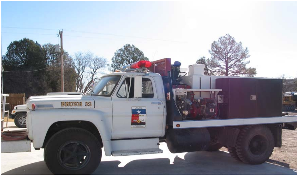
Figure 17 - 1967 Ford Brush Truck – Unknown pump size; 700 gallons of water; minimal equipment; Compressed Air Foam System (Brush 32)
