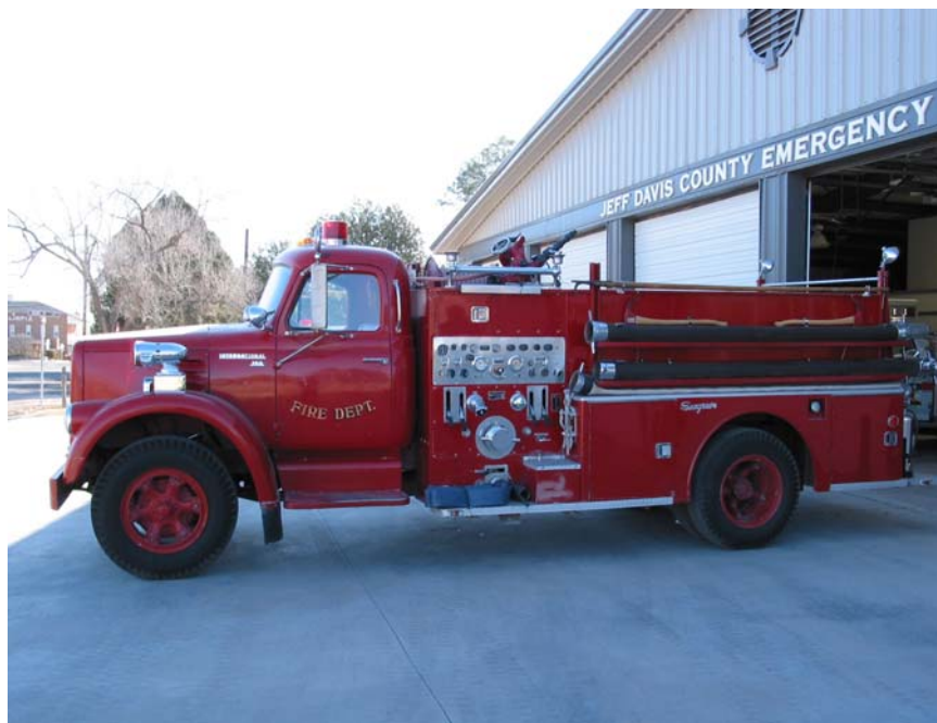
Figure 12 - 1965 Seagrave Engine – 750 GPM Pump, 500 gallons of Water, various hose, and other equipment (Engine 31)
