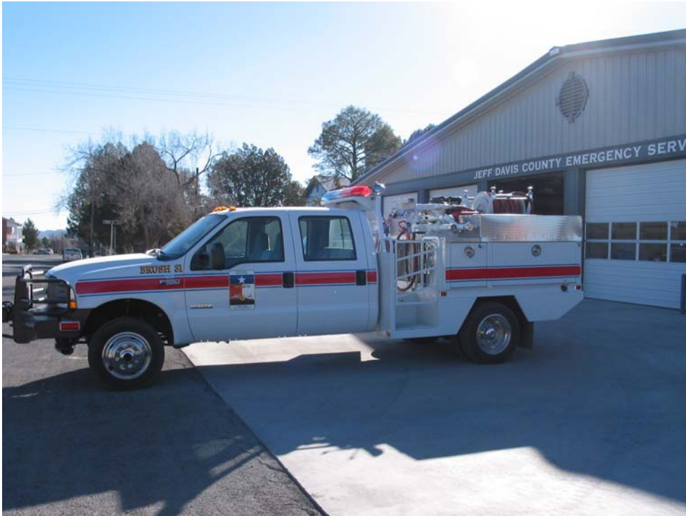
Figure 13 - 2003 Ford Brush Truck – 350 GPM Pump, 400 gallons of water, Minimal equipment (Brush 31)
