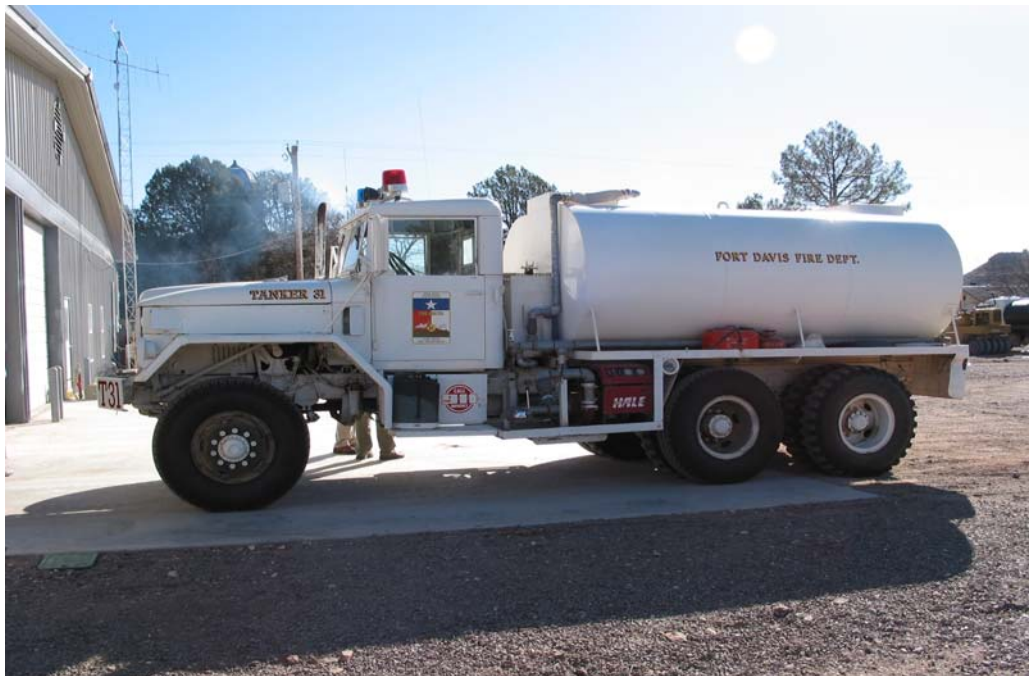
Figure 16 - 1967 GMC Tanker – 350 GPM Pump, 2700 gallons of water, Tanker 31
