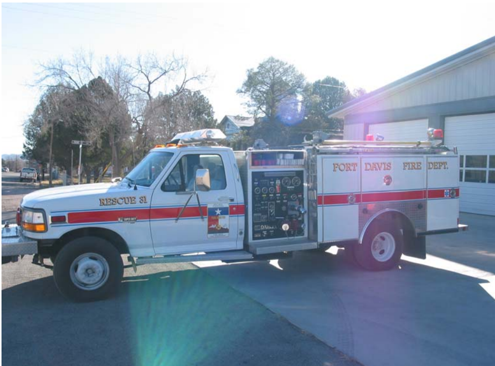
Figure 14 -1996 Ford – 350 GPM Pump, 360 gallons of Water, (Rescue 31)
