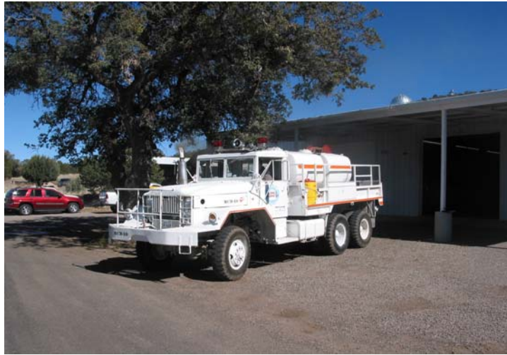
Figure 6 - Brush Truck 1 – 1979 Kaiser 5 Ton, 125GPM Pump, 1200 gallon water, 150' of pre-connected hose, Unit does carry some foam (MDC 10)
