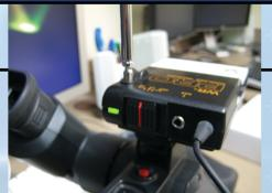
4. Switch on your wireless microphone, and set it to F1. After that, the red light on the wireless receiver will have turned green and the wireless setup is complete.
