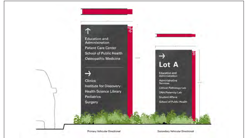
The vehicular directionals should be made up of painted aluminum sign panels with exposed aluminum red cores
