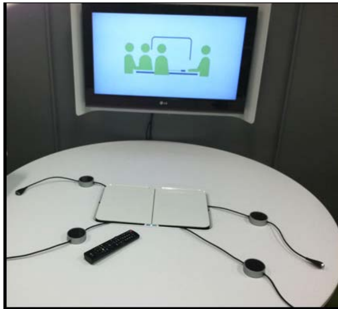
Each of the two media:scope units can accommodate up to four laptops
