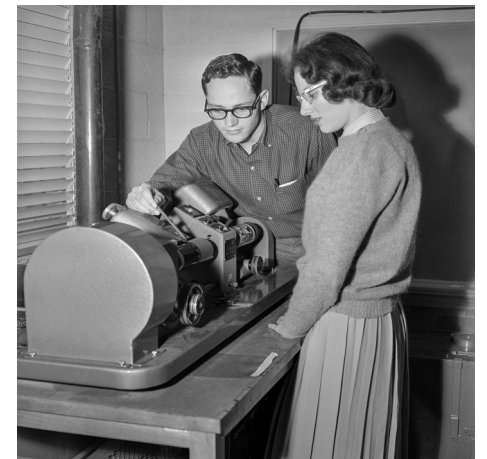
Campus Chat Editor Paul Recer shows a Fairchild Scan-A-Graver to staff member Carolyn Paine in February 1961. The equipment was used to convert photographs into engravings that were then used on a press. The equipment's capabilities allowed photographic coverage of events closer to publication deadlines.
