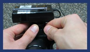
2. Check and/or replace the 9-volt batteries in the wireless receiver and microphone. When replacing the 9-volt battery, BE CAREFUL NOT TO FORCE THE BATTERY COMPARTMENT CLOSED. If it doesn't close easily, take the battery out and turn it around. Then mount the wireless receiver to the hotshoe. (Pictured above)
