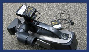
4. The side switch is used to turn the system on and off and to select a frequency. Turn on the wireless receiver to F1, the LED will light up indicating that the battery is good and the Transmitter is functioning properly. If you find the reception to be noisy on F1, change the position of the switch to F2. Make sure that the receiver is on the same frequency as the transmitter. When the LED light is green the system is working and the setup is complete.
