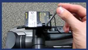
3. The "EXT MIC" input is located below the hotshoe. Now, plug the wireless receiver into the "EXT MIC" input on the camera. Next, fully extend the telescopic antenna for the best reception.
