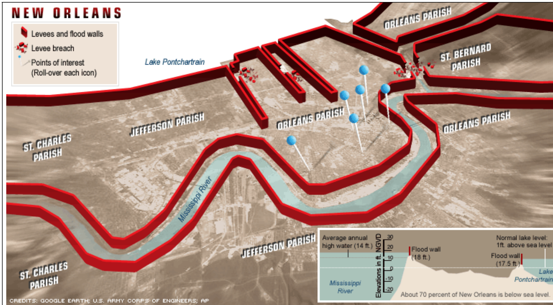
Figure 8. New Orleans levee system breaches (Source: CNN.com )
