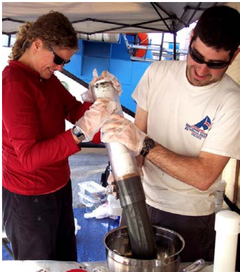
Subsurface sediment sample being "extruded" or pushed out of the tube into a stainless steel pot, where it will be thoroughly mixed before being transferred to sampling jars.
