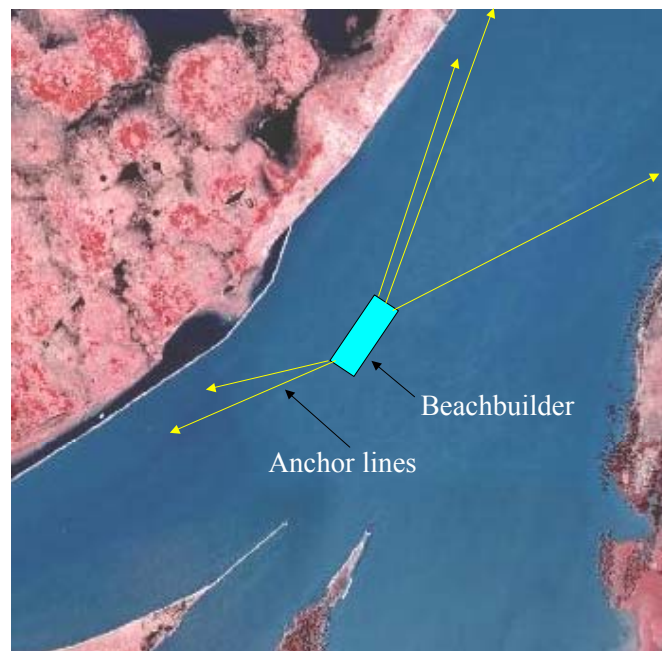
Figure 5. Initial Beachbuilder anchor deployment configuration
