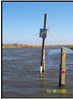
Figure 1: CRMS0434 staff gauge and continuous recorder stations. Notice the vegetation on the electrical box.
