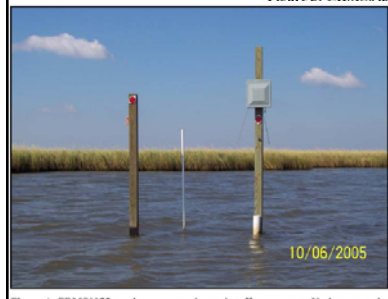
Figure 4: CRMS0375 continuous recorder and staff gauge post. Notice vegetation around the electrical box.
