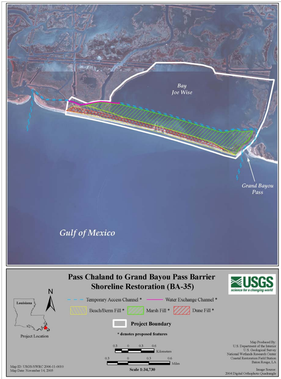
Figure 2: Phase II Project Feature and Boundary Map
