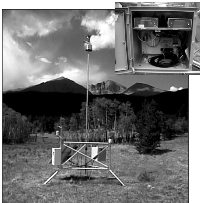
The portable air quality station was tested at Rocky Mountain National Park. The inset photograph shows the inside of the datalogger box, containing two 2B ozone analyzers and a Campbell Scientific 23X datalogger.
