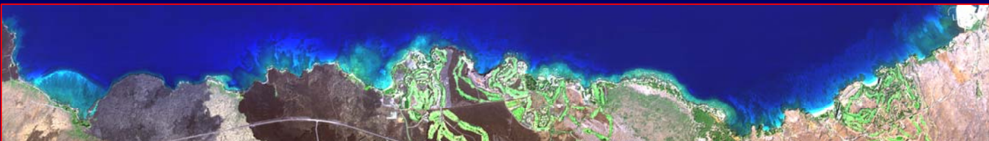
HYPERSENSPECTRAL – 72 bands between 350 and 1000 nm; 3 m pixel
