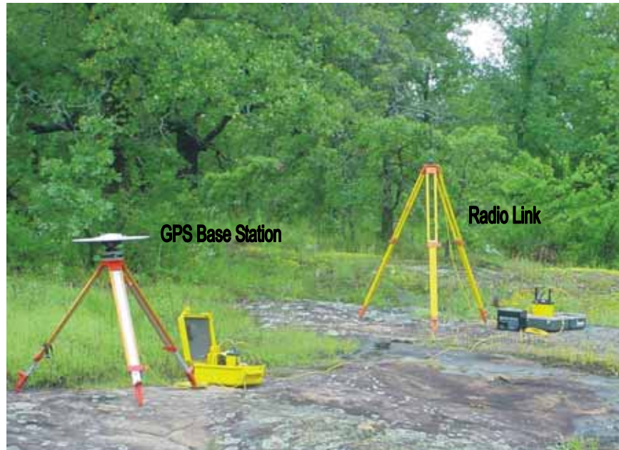
Figure 3. Base station equipment for RTK survey.
