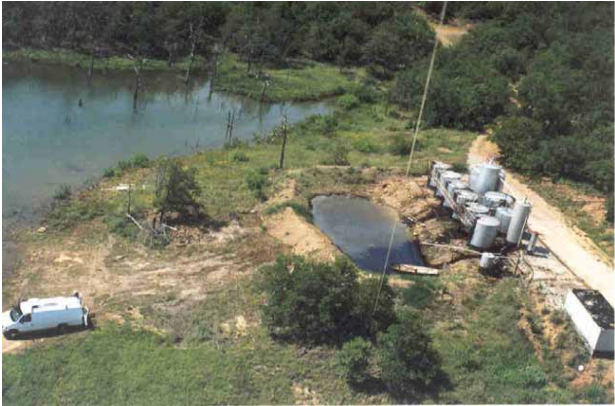
Figure 3. View of the large brine pit , the active tank battery, and the partly remediated salt scar adjacent to Skiatook Lake at the OSPER “B” site (photo courtesy of Ken Jewell, USEPA).
