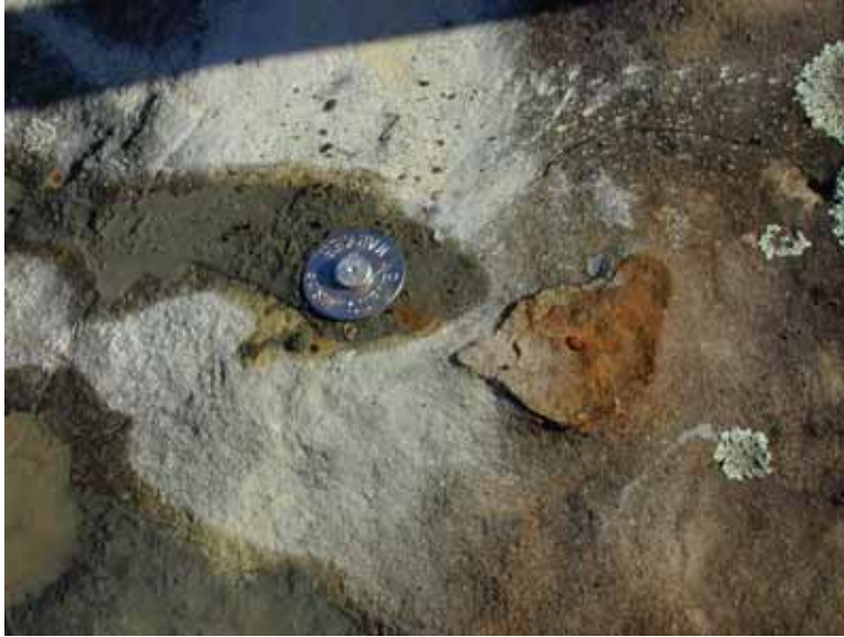
Figure 5. Monument pin used for the base station location during a RTK survey.
