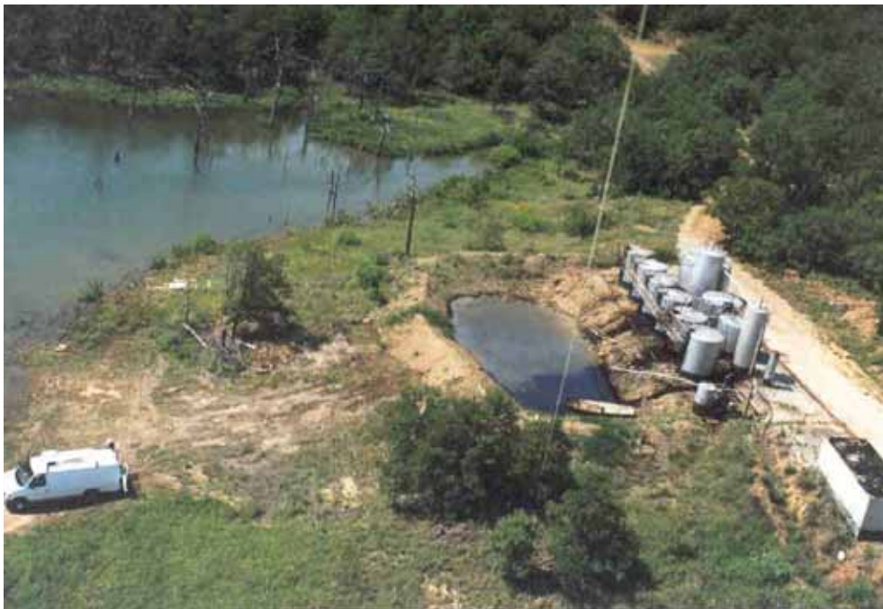
Figure 18. Aerial view of grassy area with active tank battery, pit, salt scar, and Skiatook Lake, south part of site “B.” The lake level is above the normal pool elevation. Photo by Ken Jewell, U.S. Environmental Protection Agency, Ada, Oklahoma.
