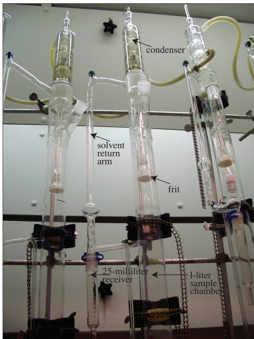
Figure 1. Continuous liquid–liquid extractors with solvent-dispersing frits mounted in a fume hood.
