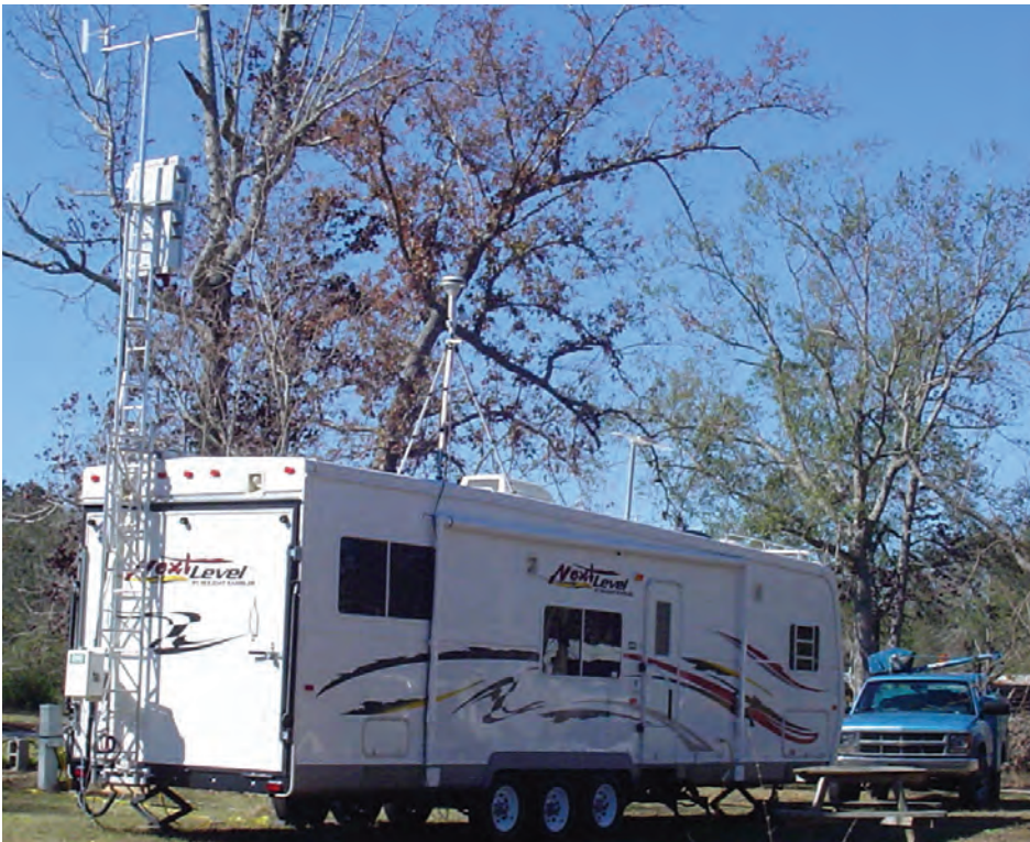
Figure 3. USGS Wisconsin Water Science Center mobile mercury laboratory deployed at Weeks Bay National Estuarine Reserve, Alabama. Instruments on mast at left rear of the trailer include the front end of the mercury speciation unit (large box) and meteorological sensors. Instrument on rooftop tripod collects fine particulate matter ( \leq 2.5 micrometers in diameter), whose mass per unit volume of air is determined by an instrument inside the trailer.
