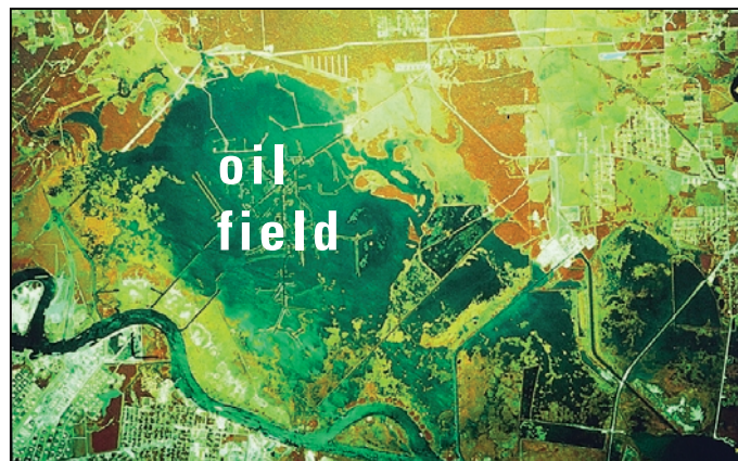
Figure 2. Air photograph of the Port Neches oil and gas field in Texas in 1978 and maps showing that wetlands above the field were healthy and continuous in 1956 but deteriorated and were converted to open water by 1978. The change was caused by induced subsidence and fault reactivation resulting from hydrocarbon production. From White and Morton (1997). Relative motion along faults: D, down; U, up.
