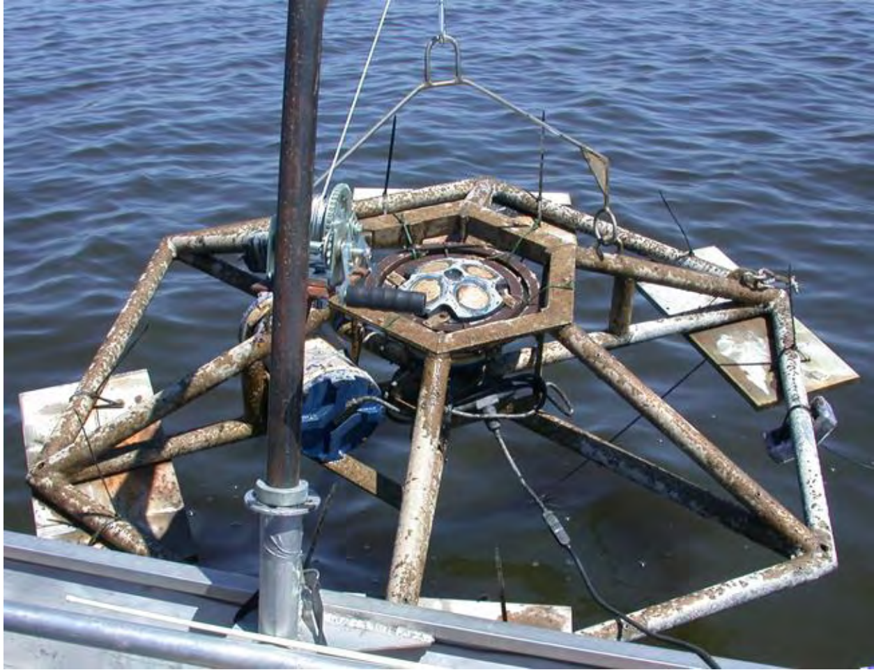
Figure 2. 600 kHz WorkHorse model acoustic Doppler current profiler shown on bottom mooring platform as deployed in Upper Klamath Lake. Onboard data measurements are being downloaded to laptop computer via cable shown in bottom right of photograph.
