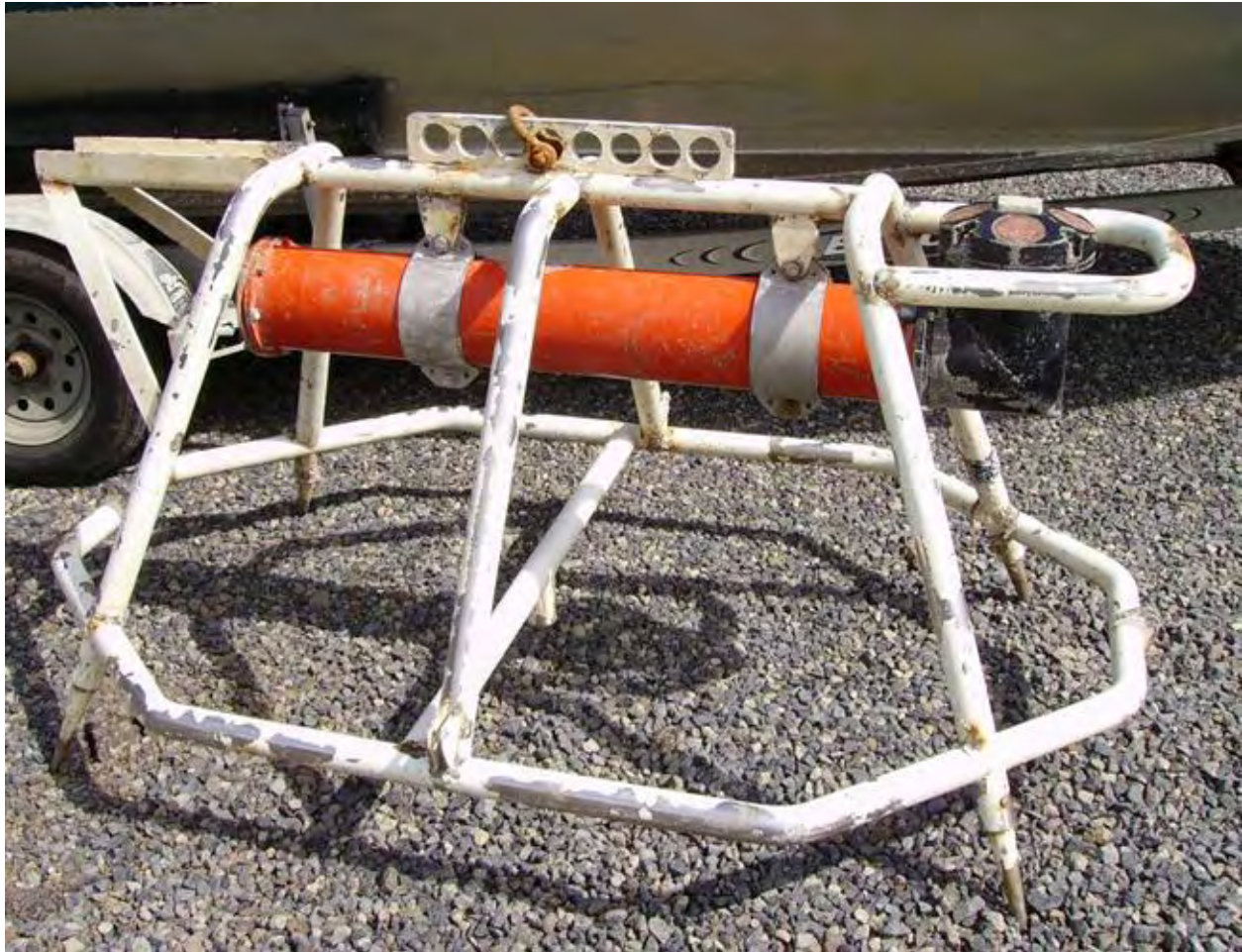
Figure 3. A 1200 kHz Broadband model acoustic Doppler current profiler on bottom mooring platform readied for deployment in Upper Klamath Lake in 2005.
