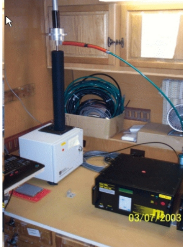
Figure 6. Photograph (a) and measurement principle schematic (b) of the TSI Aerodynamic Particle Sizer
