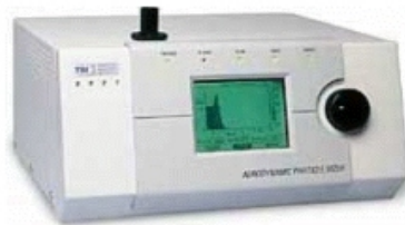
Figure 6. Photograph (a) and measurement principle schematic (b) of the TSI Aerodynamic Particle Sizer
