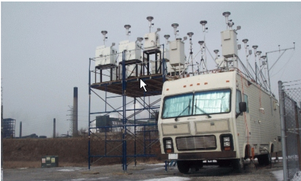
Figure 12. Photograph of the PM 10-2.5 sampler evaluation platform at the Gary, IN site.
