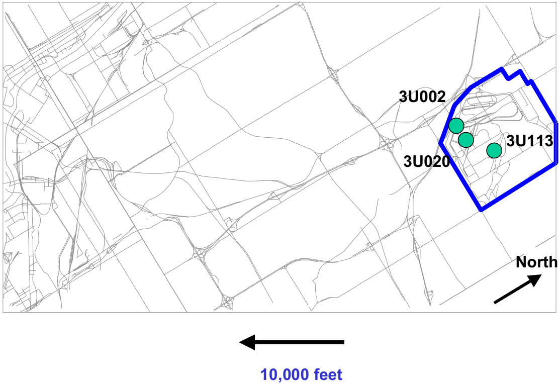
Figure 3. Panel A. Locations of monitoring wells or monitoring well clusters on the TCAAP that were involved in the geochemical study to evaluate monitored natural attenuation. Ground-water flow from right to left in the figure.
