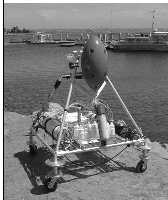
Figure 3. Benthic Flux Sampling Device 2
