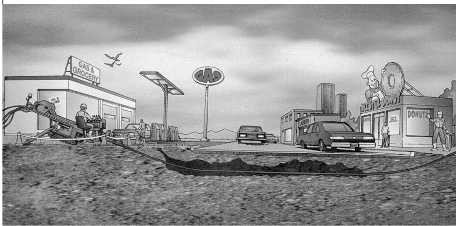
Figure 2. Installation of a Horizontal Well
