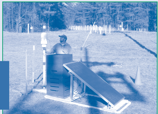
Figure 3. An SRS MicroBlower operates exclusively from power provided by a 24-volt PV panel.
