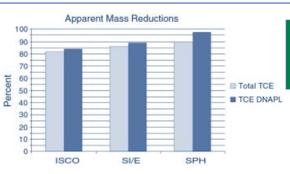
Figure 3. Apparent mass reduction estimates during the Cape Canaveral demonstration ranged from 82% to 97% based on analysis of pre- and post-soil cores.
