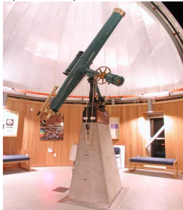
Historic 8" Alvan Clark refractor telescope is the original 1883 instrument donated by founder Anthony Chabot.
