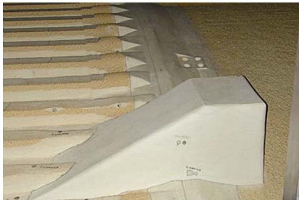
Figure 3.2-1-2. ET forward bipod ramp (foam).
