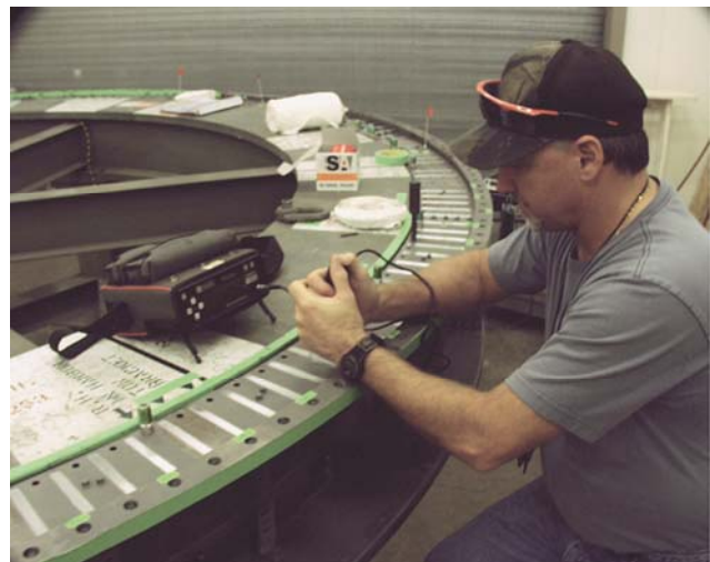
Figure O10.10-1-3. Harness testing.
