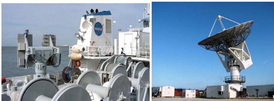
Figure SSP 12-1. X-band radar on solid rocket booster recovery ship (left), MCR C-band radar (right).
