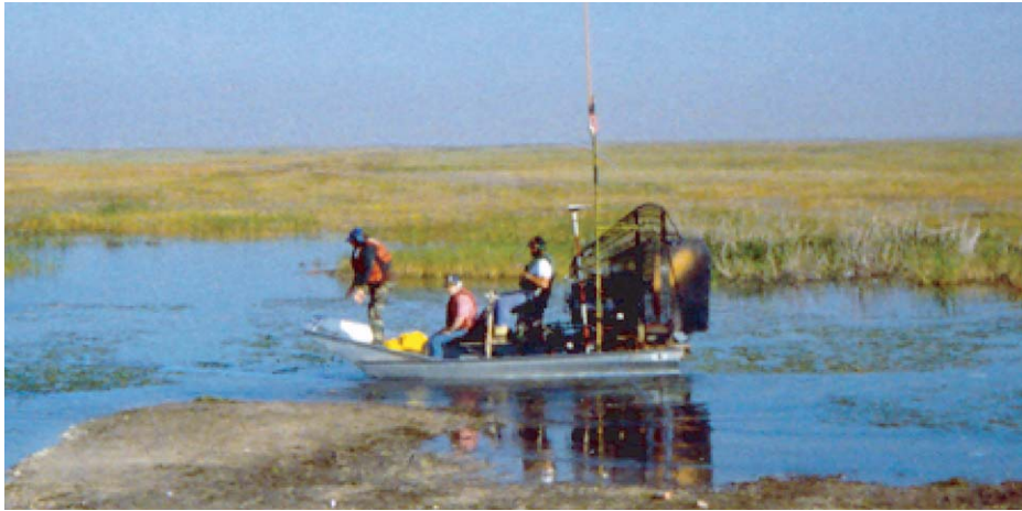
Figure 2. Airboat configured for collecting GPS data launching for a surveying session.
