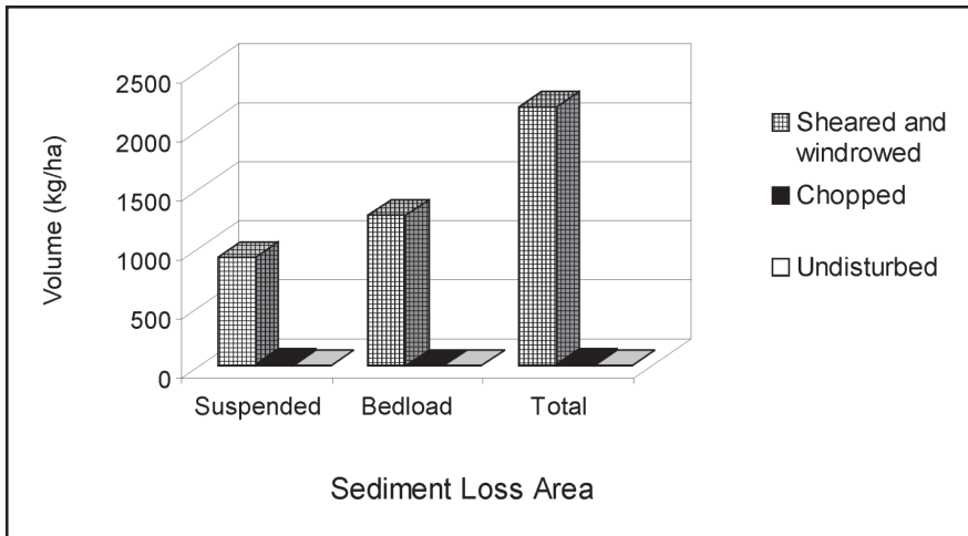
Figure 3-41. Sediment loss (kg/ha) in stormflow by site treatment from January 1, to August 31, 1981 (TX) (after Blackburn et al., 1982).
