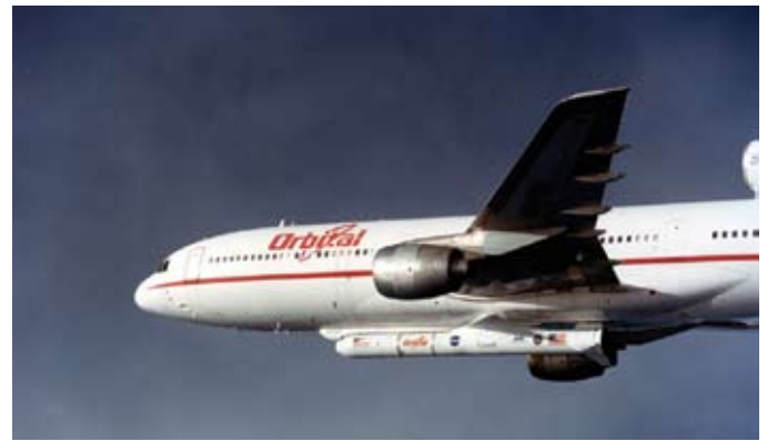
The L-1011 carrier aircraft is in flight with its cargo of the Pegasus launch vehicle and SciSat-1 spacecraft underneath.
