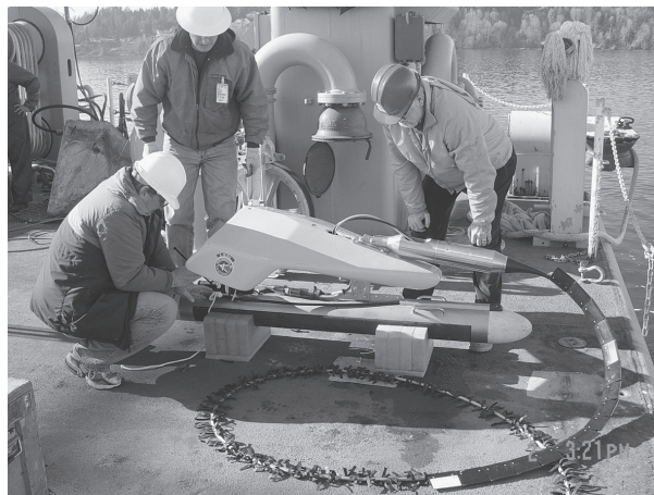
Figure 2. Sidescan sonar being prepared for launch during sea trials in Puget Sound. Photo by Doug Swain.
