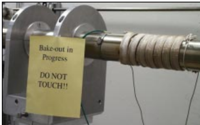
A correctly grounded heater tape in use to dry a section of beam pipe.
