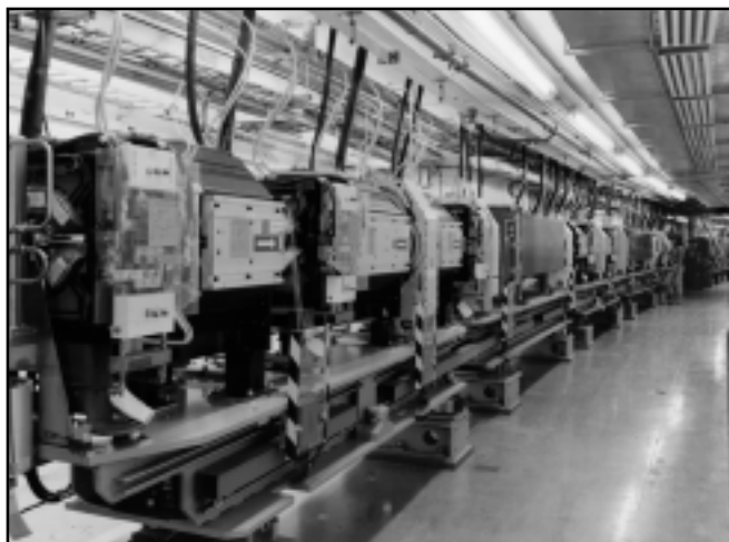
The 1104-meter circumference storage ring steers and focuses the beam using 1097 electromagnets.
