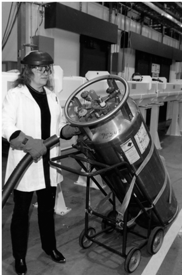
Debra Hilborn of IMCA-CAT works with a portable dewar that could be made obsolete with the advent of a centralized liquid nitrogen system.
