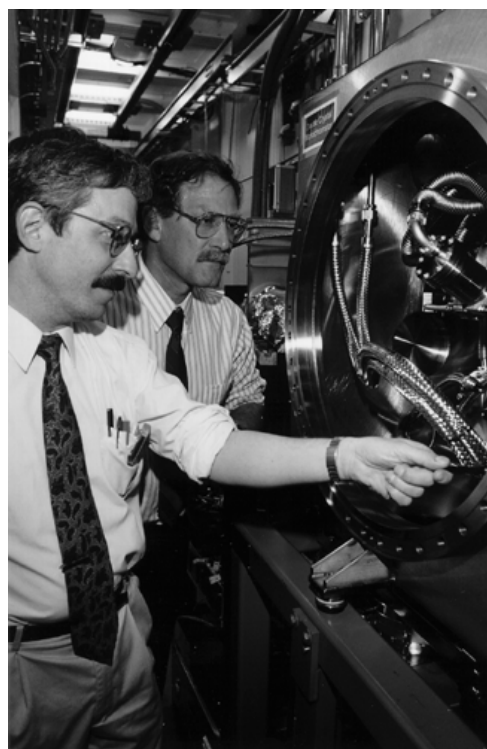
Jon Tischler and Gene Ice inspect the double crystal monochromator at UNI-CAT's 33-ID.
