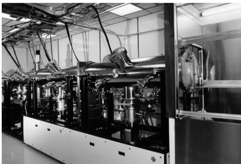
The 1.5m sputter-deposition facility in the APS-ML.
