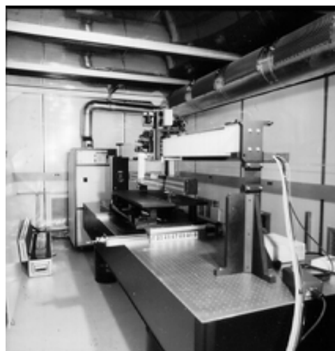
The Long Trace Profiler (LTP) is used to measure slope and curvature of optical surfaces.
