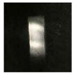
Direct film exposure of the SPPS x-ray beam in the experimental hutch. (Courtesy of Stanford Synchrotron Radiation Laboratory)
