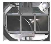
The SPPS multilayer monochromator designed and fabricated at the APS. (Courtesy of Stanford Synchrotron Radiation Laboratory)
