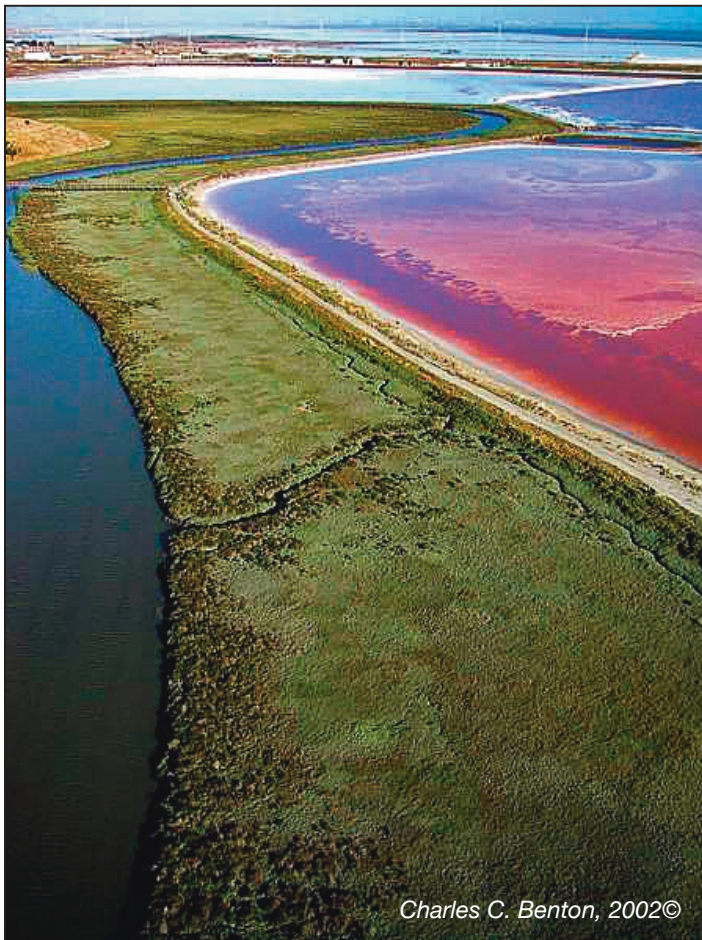
Levees that divide salt ponds from neighboring sloughs also help control flood waters.
