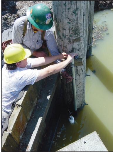
USGS scientists servicing a salinity and temperature probe in a pond. Installed sensors continually measure water quality parameters in select ponds.
