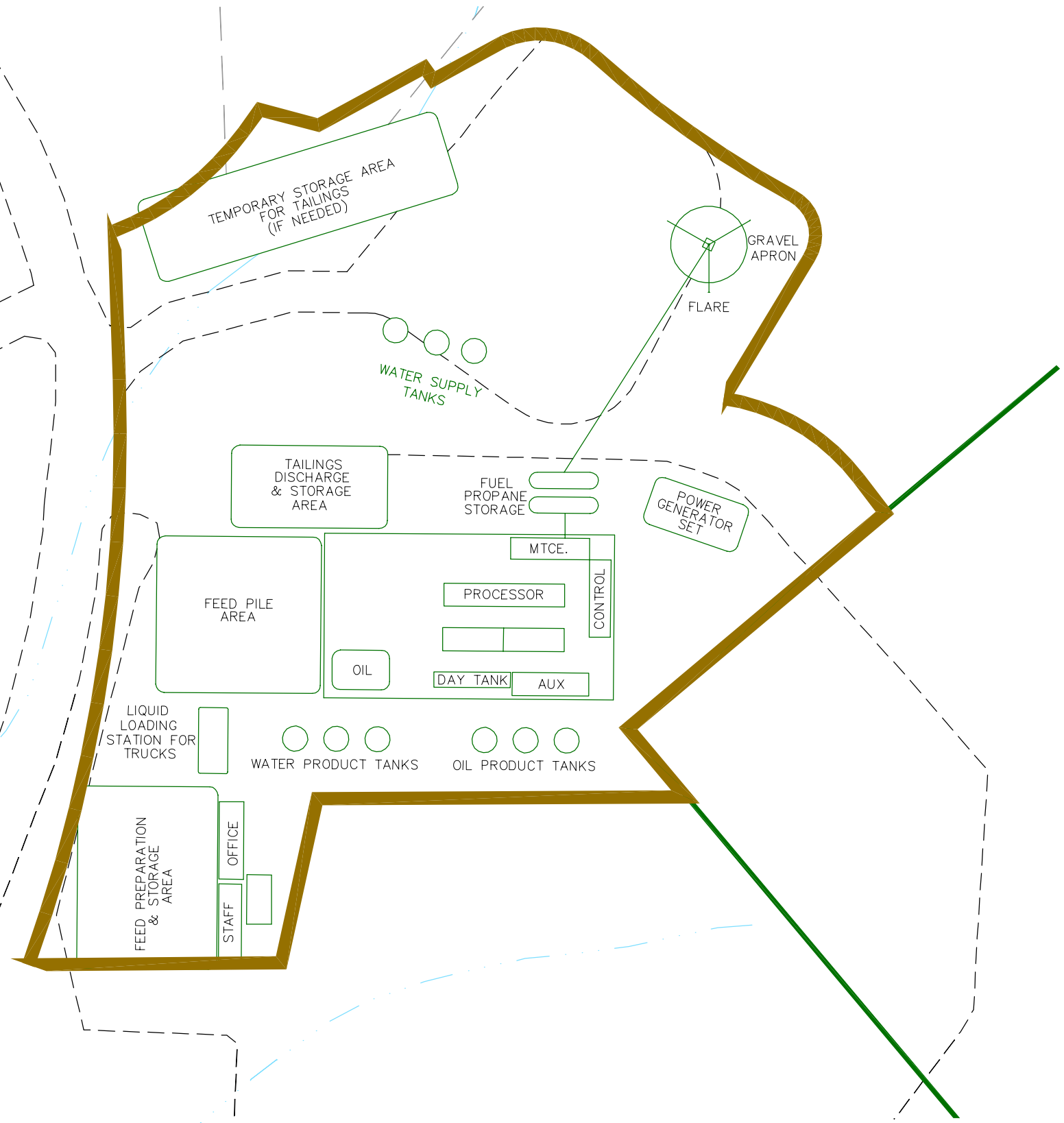
SITE LAYOUT GENERAL ARRANGEMENT PHASE 2 PROCESSING PLANT WHITE RIVER LEASE AREA, UINTAH COUNTY, UTAH
