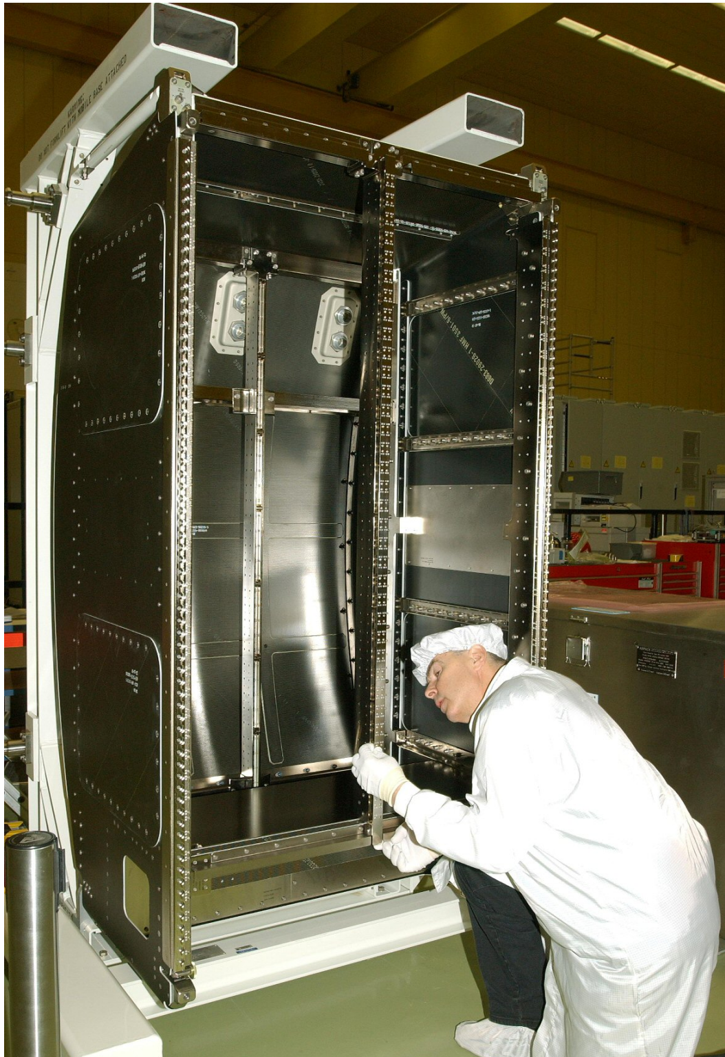
International Standard Payload Rack into which experiment facilities, subsystems or storage racks can be fitted. (Image: EADS Astrium)
