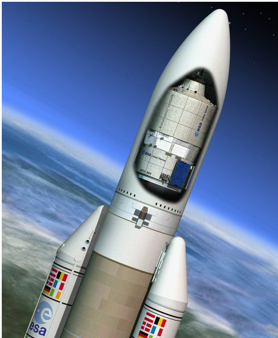
The ATV enclosed in Ariane's protective fairing during launch phase (Image: ESA/D.Ducros)
