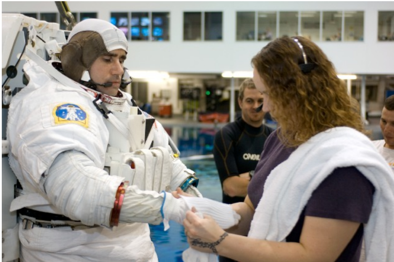
Cosmonaut Yuri I. Malenchenko, Expedition 16 flight engineer representing Russia's Federal Space Agency, dons a training version of the Extravehicular Mobility Unit (EMU) space suit prior to being submerged in the waters of the Neutral Buoyancy Laboratory (NBL) near the Johnson Space Center. Suit technicians assisted Malenchenko.
