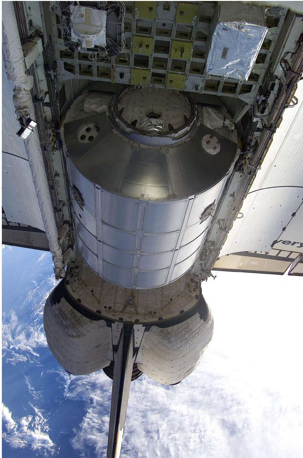
Multi-purpose Logistics Module 'Leonardo' in the space shuttle cargo bay on March 10, 2001, during the STS-102 mission to the ISS. The Columbus Laboratory shares its basic structure with the Multi-Purpose Logistics Modules. (Image: NASA)
