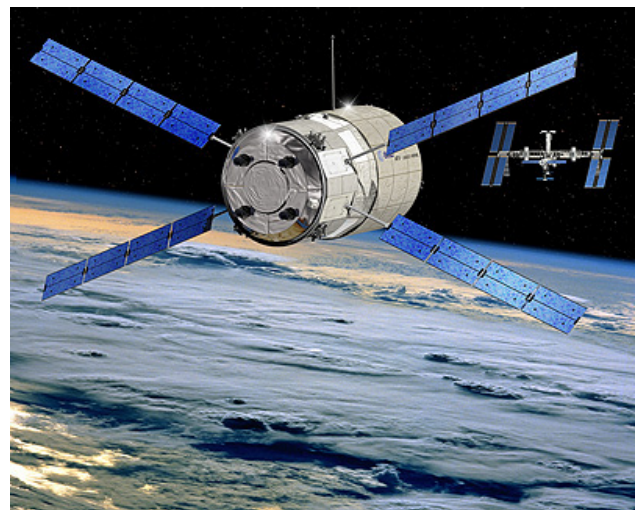
Artist's rendition of the Automated Transfer Vehicle approaching the International Space Station.
