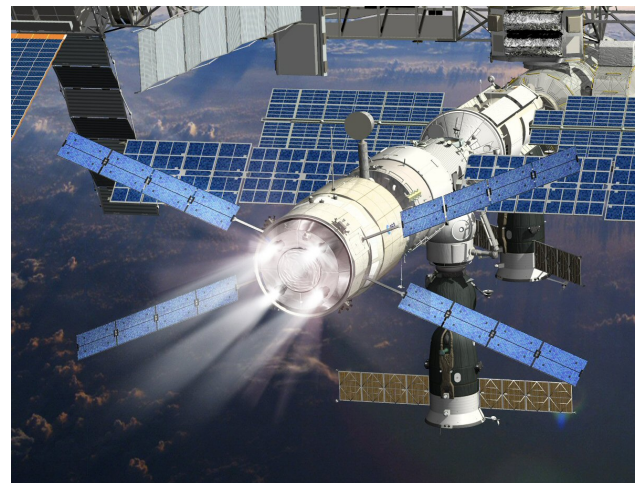
The ATV will be used to raise the altitude of the ISS (Image: ESA/D.Ducros)
