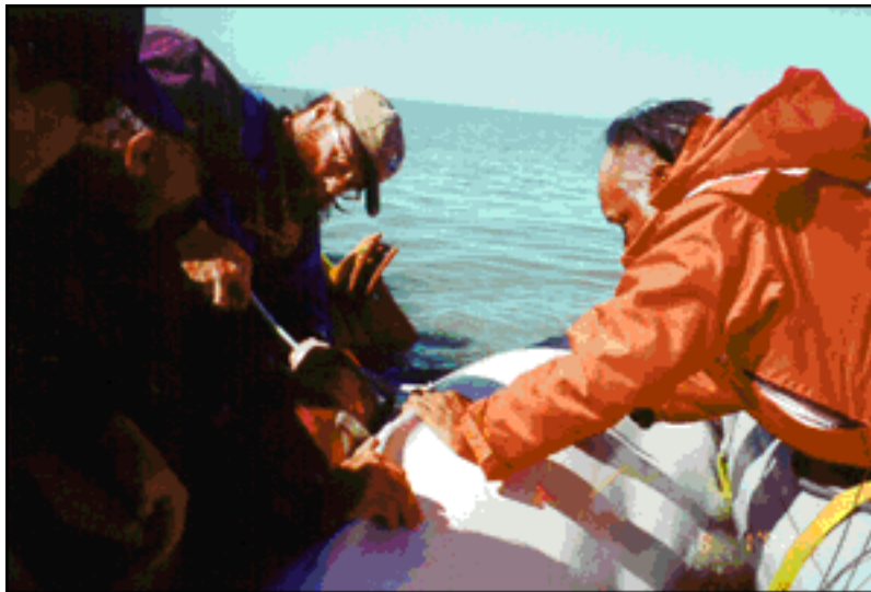
Tagging: NOAA researchers and Native subsistence hunters work together to attach tags. Here 3/8" pins are inserted into the skin and blubber of the whale to hold the tag.
