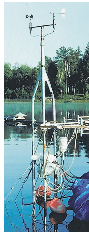
A stable tower anchored to the bottom of Williams Lake is one of the few sites where water evaporation and carbon dioxide flux have been directly measured over a lake.
