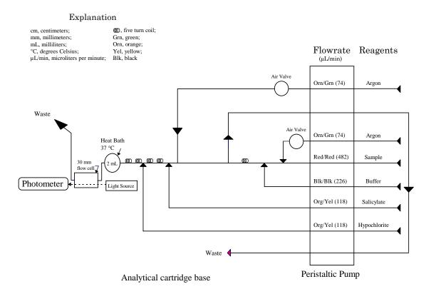
Figure 3. The flow regime used for the analysis of ammonium
