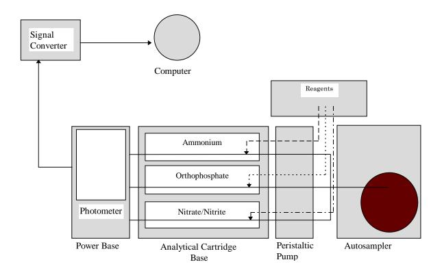
Figure 1. Schematic of automated nutrient analysis equipment.
