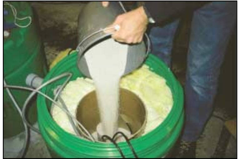
Figure 10a. Pouring sand around seismometers
