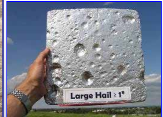
Aluminum foil-wrapped Styrofoam hail pads
