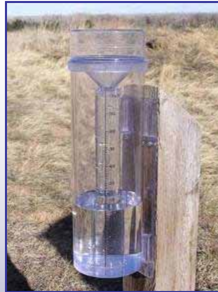
4-inch diameter high capacity rain gauges
