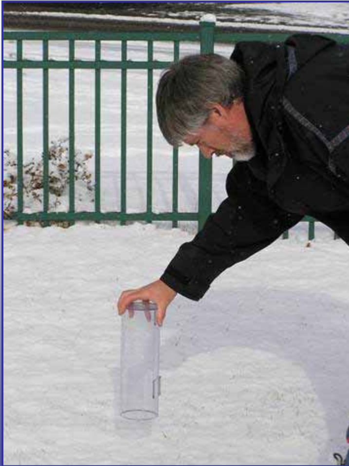
Place gauge upside down and push down into the snow
