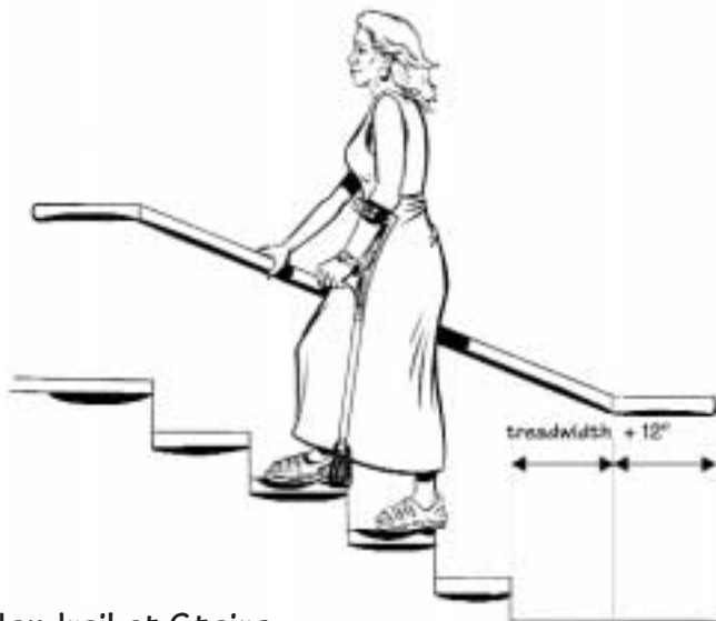
Handrail at Stairs
