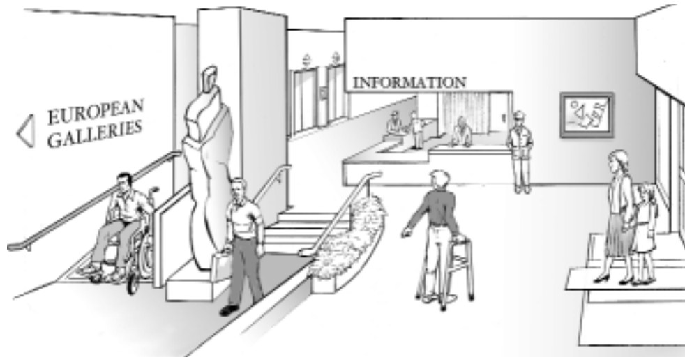
Interior Accessible Route
