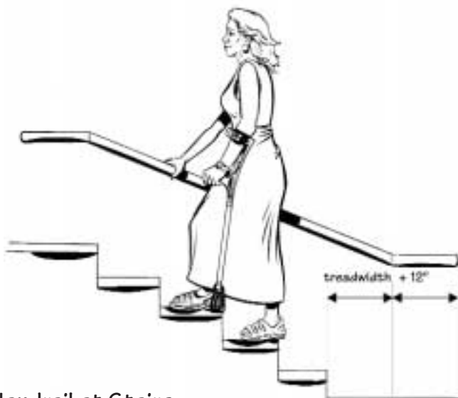
Handrail at Stairs
